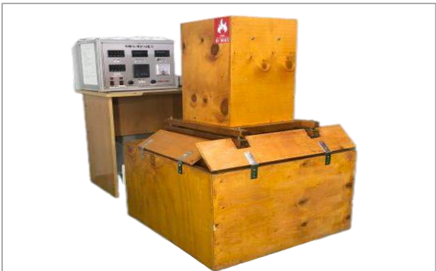
INCREASED HEAT DETECTOR TEST MACHINE
