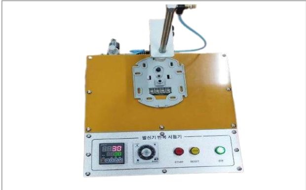
MACHINE TO TEST THE RELIABILITY OF THE FIRE ALARM BUTTON
