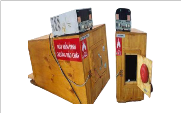
BELL FIRE ALARM TEST MACHINE
