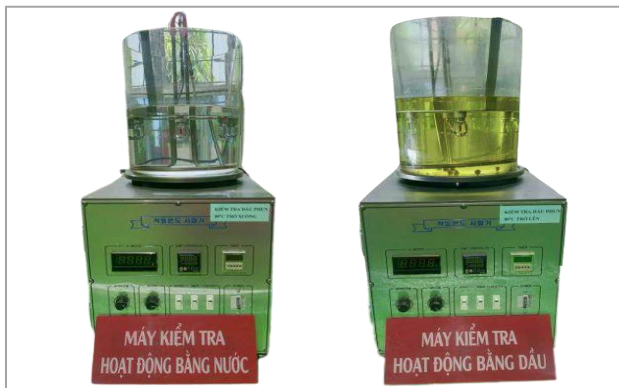
MACHINE TO CHECK SPRAY HEAD OPERATION
