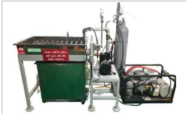
INJECTOR LEAK PRESSURE TEST MACHINE
