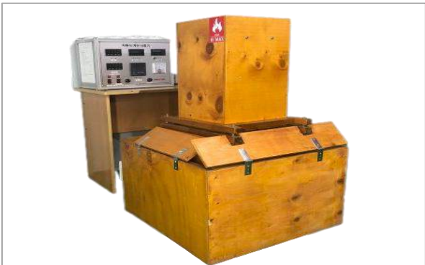
INCREASED HEAT DETECTOR TEST MACHINE
