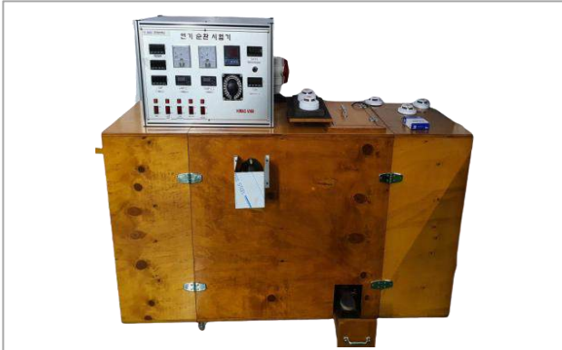
PHOTO ELECTRIC SMOKE DETECTOR TEST MACHINE
