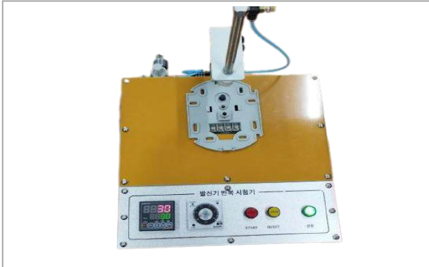
MACHINE TO TEST THE RELIABILITY OF THE FIRE ALARM BUTTON
